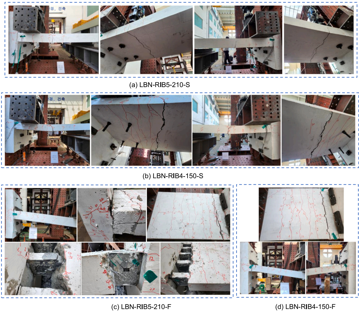
Fig. 8. Failure mode of experimental specimens.
